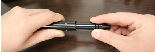
Figure 2.1. To install the electrode, first remove the Stylus Shaft (A) from the Stylus Hull (E) by pulling them apart.
