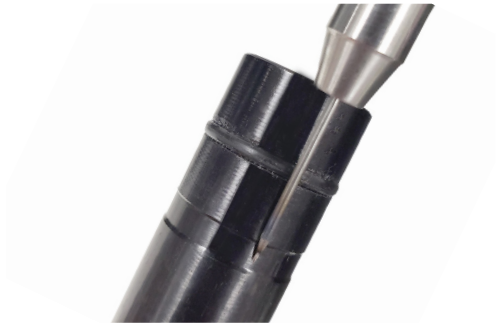
Figure 2.2. Use the guide on the side of the Stylus Hull (E) for proper Electrode (D) positioning.
