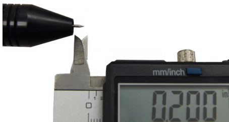
Figure 2.3. Electrodes should protrude past the stylus hull 1/8 to 1/4 inch (3.175 to 6.35mm).
