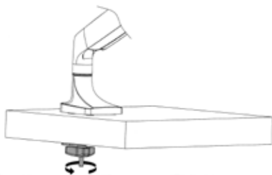
Figure 4.1. Turn the Adjustment knob (J) clockwise to tighten the plate to the table.
