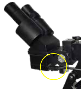
Figure 5.1 After installing the rubber eyepiece covers, use the RJ45 Shutter Cable to connect the welder to the back and bottom of the microscope head. The other end of the cable connects to the (F) port in the back of the Orion PJ. (See Figure 2.1)
