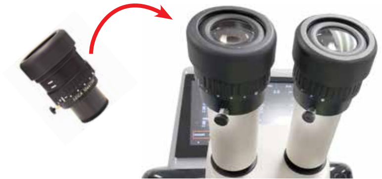
Figure 9.1 Attach eyepieces to the microscope tubes and tighten the screws with an Allen wrench. The eyepiece with the crosshairs is attached to the right tube.
