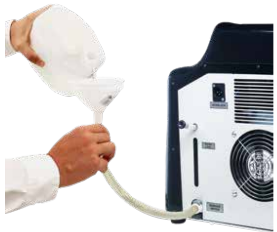
Figure 9.2. To fill the welder with coolant water, attach the funnel, tube, and connector to the bottom Female Connector "Remove Water" Port. Remove the Red Plug from the Upper Connector tube. Fill the welder with deionized water that comes with the Orion LZR laser welder.
