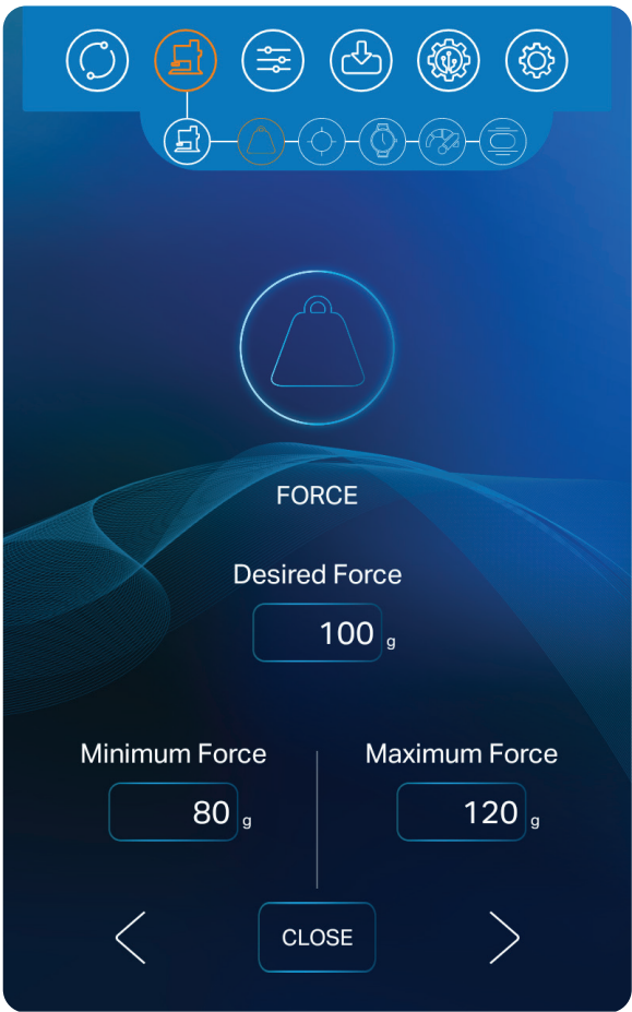
Figure 15.1. Select the desired amount of force to be delivered by the weld head in the Force Screen, the second weld head setup step.
