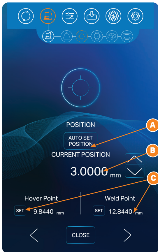
Figure 16.1. Setting the position is the third step in the setup process. Press the Auto Set Position Button A) to automatically set the Hover Point and Weld Point. You can manually adjust these points by pressing Hover or Weld Point Set Buttons (C).. Be sure to touch the Set Buttons once the desired position is achieved to establish the points.
