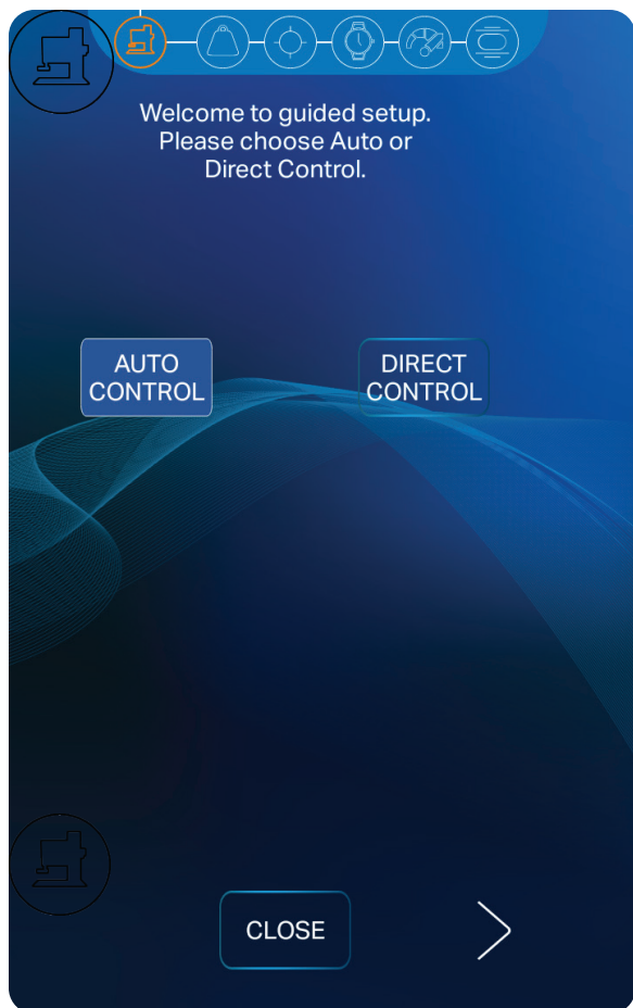
Figure 14.1. The Weld Head Control Screen in the Mode Select step. When you touch the Weld Head Control Screen icon, the Pico will want to walk you through a step-by-step process to complete the weld head setup process. When you've selected the desired settings for each step, press the right arrow button at the bottom of the screen to advance to the next step. You can press the left arrow button to go back. Press the Close button to save and end the setup process.
