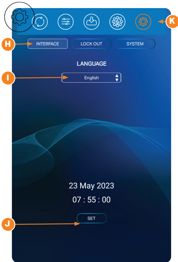
Figure 28.1. Use the Settings Screen to make changes to the Pico's general system settings, such as language, defaults, Wi-Fi, and locks.
