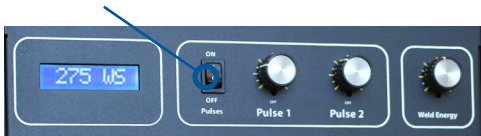
Figure 8.2. When using a Roll Spot hand held attachment, be sure the Pulse setting is on.
